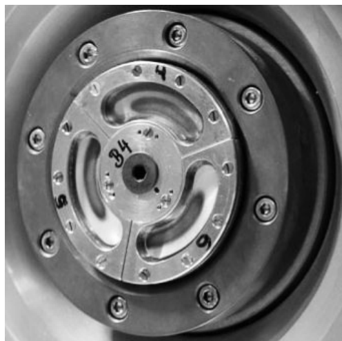
Figure 3. The GSI rotating target wheel.
