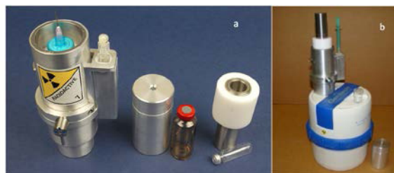
Fig. 1. Radioisotope concentrator device with standard accessories (a) and the radioisotope concentrator device coupled with ^{99m}\text{Tc} generator for in-line elution/concentration of ^{99m}\text{Tc} eluate (b).
