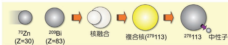
Fig. 4 The figure shows the reaction scheme for the ^{70}\text{Zn} + ^{209}\text{Bi} . The experiment was designed to produce the isotope, ^{278}113 , by the one-neutron evaporation.
