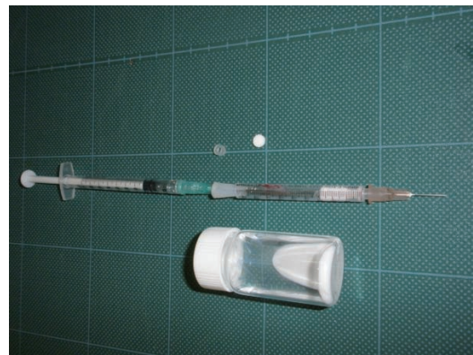
Fig. 1 Manufactured generator assembly with its parts. From bottom to up: adsorbent \text{SnO}_2 powder (before \text{HNO}_3 treatment); generator connected with eluent syringe; and porous plastic diskette and short end of plastic tube (See text for more detail).
