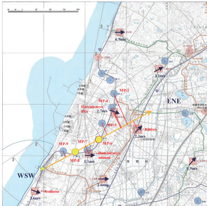
Fig. 5 Estimated course of thunderclouds on Apr. 8, 2018. Yellow arrow : Estimated course of thunderclouds Red line : Perpendicular to course of thunderclouds from monitoring posts Yellow star : Estimated radiation starting point (268 m from the coastline) Wind direction and wind velocity : Average value (6:50 ~ 7:00) at 13 m above the ground
